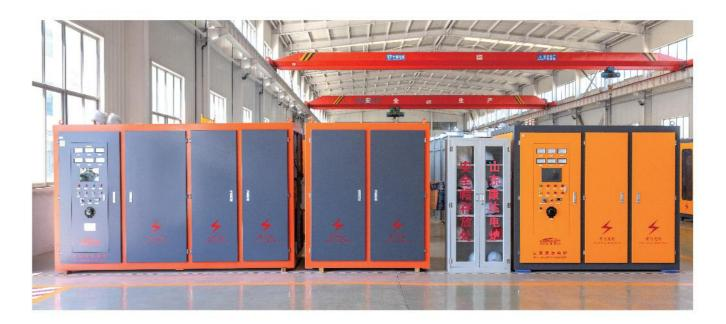
The KGCL series intermediate frequency power supply, developed by Kangda Electric Furnace, adeptly handles the one-to-two (or one-to-many) operating mode. It facilitates a melting process that involves melting in one operation while maintaining heat in another (or multiple melting operations with multiple heat maintenance). This can greatly improve the utilization rate of transformers and achieve maximum efficiency.
